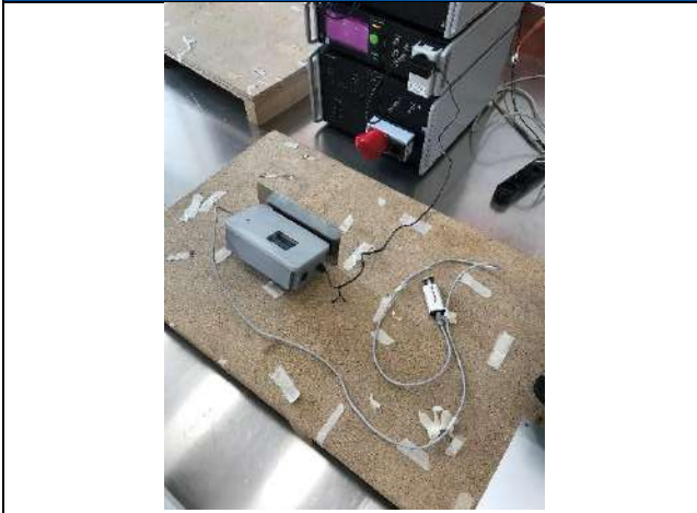
PHOTO 5 – BURST/SURGE/DIPS IMMUNITY SETUP
