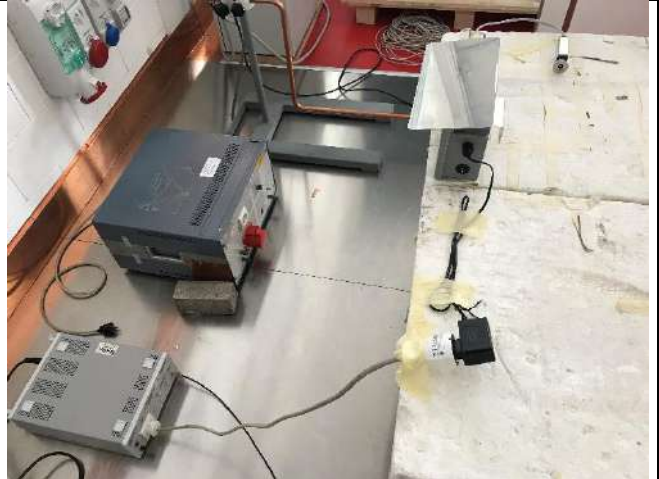
PHOTO 3 – CONDUCTED EMISSIONS DISTURBANCES
