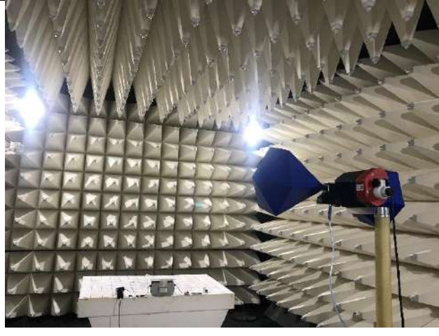
PHOTO 2 – RADIATED EMISSIONS DISTURBANCES
