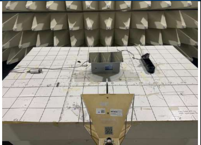
PHOTO 4 – RADIATED IMMUNITY SETUP
